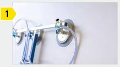
Six powerful suction pads with sensing valve for panel transport.
