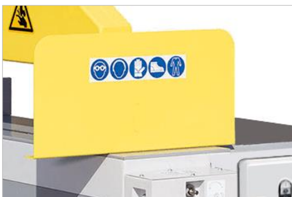
Figure 33: protective shield (standard version)
