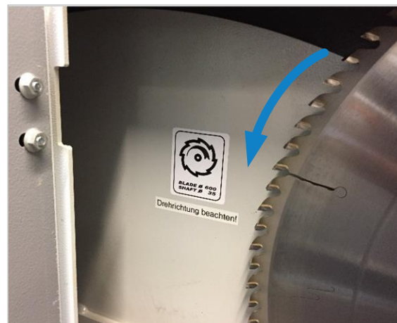
Figure 30: direction of rotation of the saw blade
