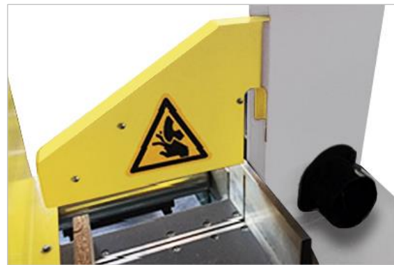
Figure 32: clamping guard for model UTK 350
