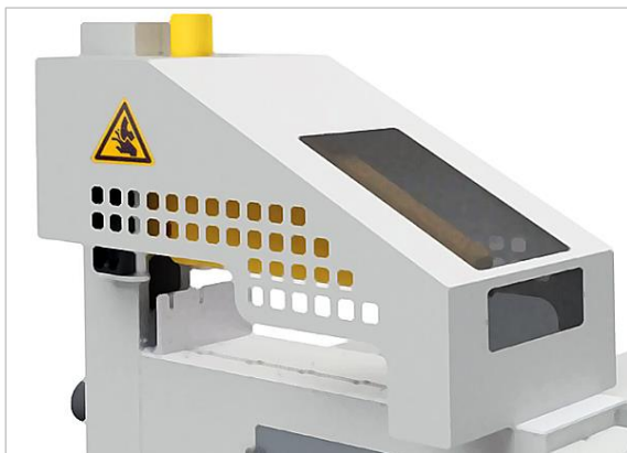
Figure 35: full protection cover with viewing window
