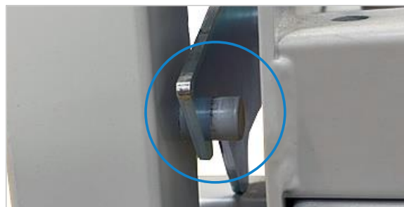
Figure 10: Swivel frame is engaged vertically
