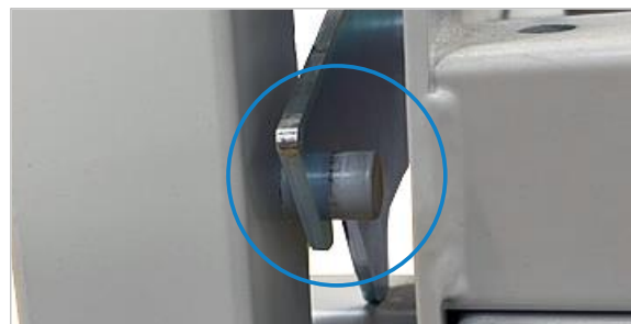
Figure 10: Swivel frame is engaged vertically
