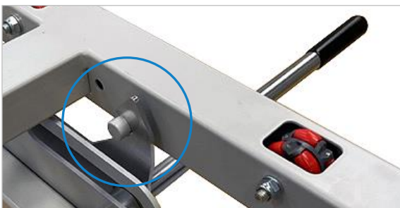
Figure 9: Swivel frame is engaged horizontally
