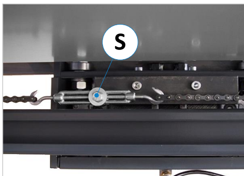
Figure 13: Fitting and tensioning the link chain
